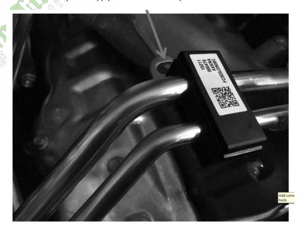
\*\*NOTE\*\*: Before proceeding, carefully clean the top of the high pressure pump and surrounding areas to remove any loose dirt or debris as it is critical no contamination finds its way into the fuel system. This step can be dismissed at your own risk. When working with fuel systems, cleanliness is an absolute must.
