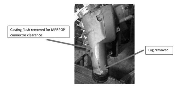
The casting flash rib in the area shown above should be removed to avoid interference with the MProp connector when the manifold is reinstalled.
