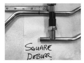
These hardline assemblies are readily available from Ford so if you wish, you can purchase the hardline feed and return assembly for modification. This will provide a clean feed line to modify as well as new o-rings for the adapter block.
