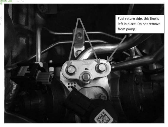
Remove the "T-bar" shown in the picture above stamped "FoMoCo" by loosening the 10mm flanged head bolt. This bolt will be reused to attach the failsafe adapter.
