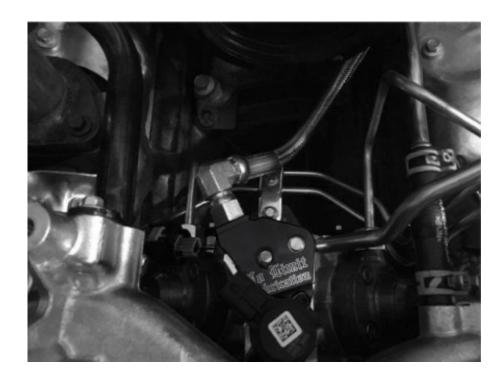
Note: This 2 wire braided hydraulic line must not touch any component as it is fit into the valley and run out.
