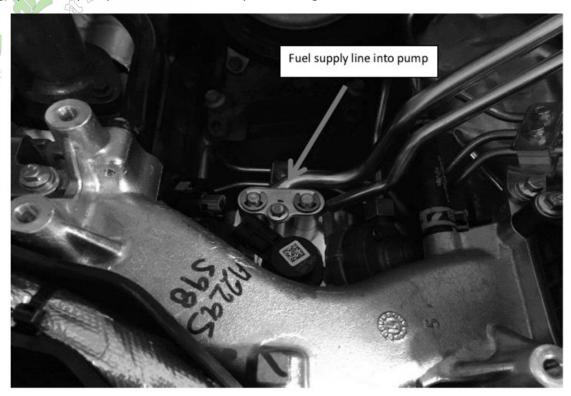
Removal of the fuel filter and fuel filter base housing is required to gain clearance to remove the upper plastic air manifold. Remove the hard plastic line from the filter to the fuel supply steel line that goes to the high pressure pump. The supply line to the pump is on the passenger side of the pump. See image above.
