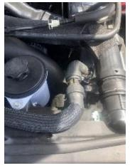
9) Now that the intercooler is installed and all the bolts and clamps are tight make sure you close the drain on the radiator. Then you can reinstall the battery and refill the secondary system on the passenger side fan shroud.
