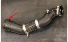
Twist carefully (1/4 turn counter-clockwise) to unlock and remove the intake air temperature sensor from the factory plastic throttle body coupler. Apply some vaseline or grease to the o-ring of the factory intake air temperature sensor and install it into the machined port on the supplied HSM billet aluminum throttle coupler. Be sure to carefully twist the sensor to properly lock it into place (1/4 turn clockwise).
