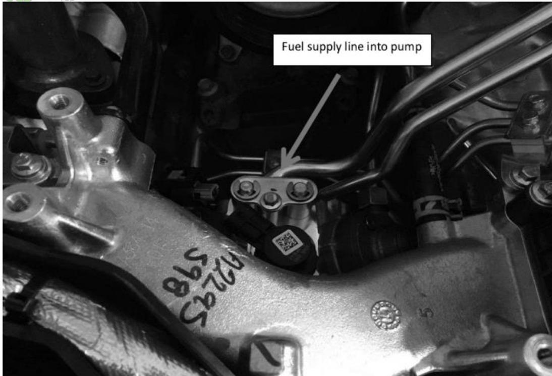
Removal of the fuel filter and fuel filter base housing is required to gain clearance to remove the upper plastic air manifold. Remove the hard plastic line from the filter to the fuel supply steel line that goes to the high pressure pump. The supply line to the pump is on the passenger side of the pump. See image above.
