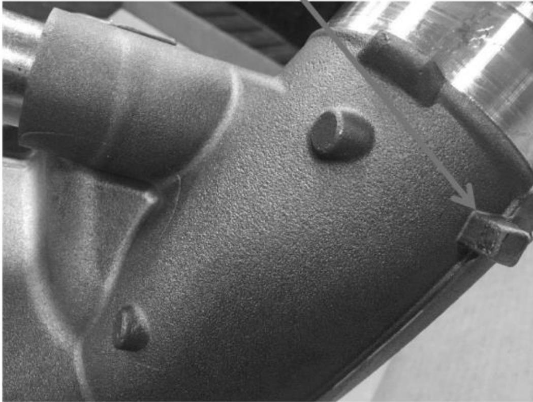
Casting flash removed for MPRPOP connector clearance
