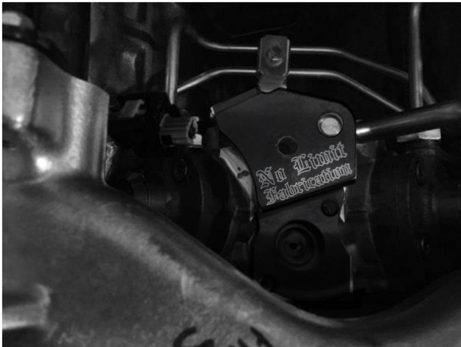
Install metering unit and tighten all fasteners.
