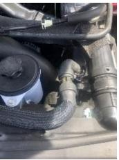
9) Now that the intercooler is installed and all the bolts and clamps are tight make sure you close the drain on the radiator. Then you can reinstall the battery and refill the secondary system on the passenger side fan shroud.
