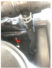
3) Once you have the battery removed you can then remove the (2) 13mm bolts that mount the intercooler to the battery tray.
