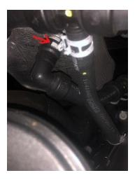
5) Once the intercooler is removed you can then begin modifying the coolant lines. On the 2011-2016 trucks you will have grey spring clamps and the 2017-2020 trucks will have a plastic crush ring
