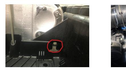
4) Then once the coolant has fully drained you can pull the Upper Radiator Hose and black quick connect fitting with the white squeeze tabs off the intercooler and you can pull the old intercooler out of the truck.
